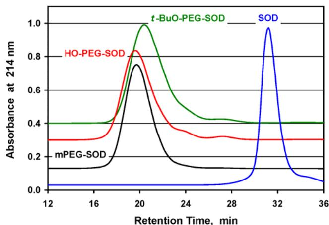
**Figure S3.** Size-exclusion chromatography of superoxide dismutase (SOD) and of conjugates with 10 kDa HO-PEG, mPEG and *t*-BuO-PEG containing an average of c. 2-3 molecules of PEG per SOD subunit. The Superdex 200 column was eluted with 10 mM sodium carbonate buffer, pH 10.1, containing 100 mM NaCl at a flow rate of 0.5 mL/min.
