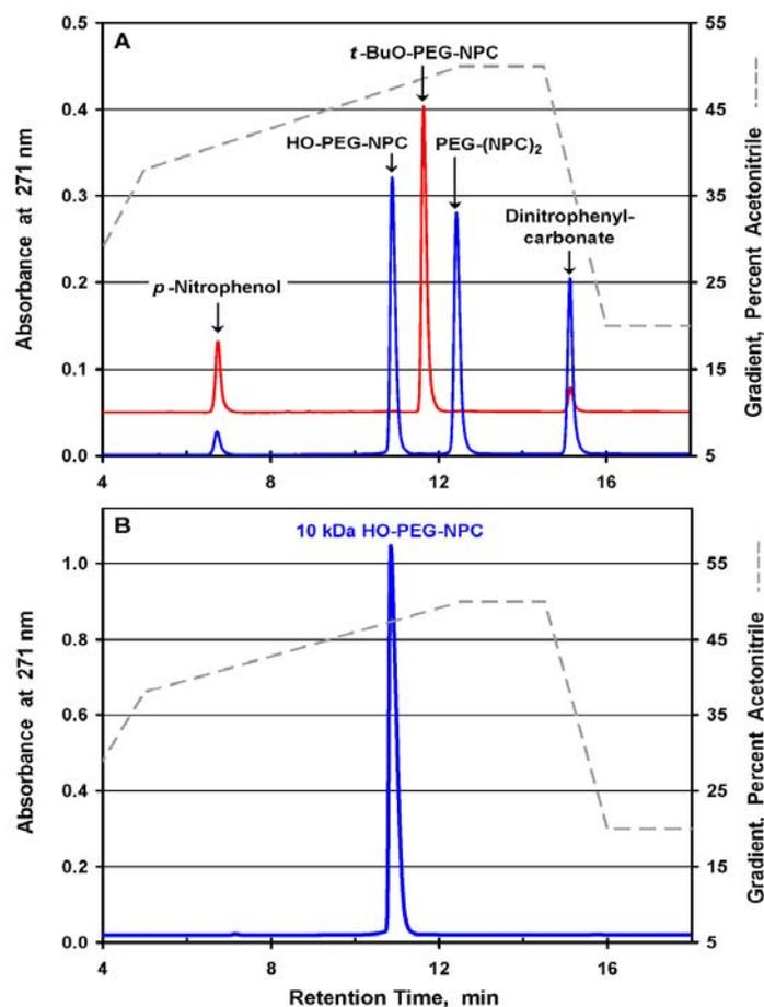
**Figure S2.** Analytical reversed-phase chromatography of reaction mixtures for synthesis of 10 kDa HO-PEG-NPC and *t*-BuO-PEG-NPC (A) and of purified HO-PEG-NPC (B) on a Jupiter C4 column (4.6 x 150 mm), with a dog-leg gradient of 20% to 38% to 50% (v/v) acetonitrile containing 1 mM HCl. Absorbance was monitored at 271 nm, the absorbance maximum of the *p*-nitrophenylcarbonate group.
