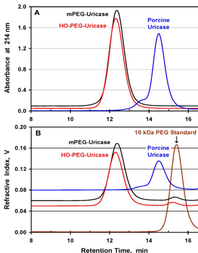
**Figure S6.** Size-exclusion chromatography of porcine uricase and of conjugates containing an average of c. 2-3 molecules of 10 kDa mPEG or 10 kDa HO-PEG per uricase subunit on a TSK G-5000PW<sub>XL</sub> column in 10 mM sodium carbonate buffer, pH 10.1, containing 100 mM NaCl, at a flow rate of 0.6 mL/min. The retention times of the refractive index signals (panel B) were corrected for the 0.25 minute lag between the absorbance detector and the RI detector.
