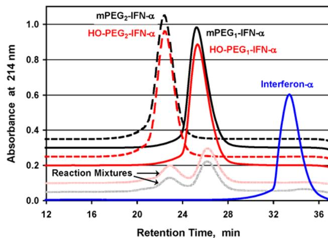
**Figure S4.** Size-exclusion chromatography of interferon- $\alpha$  starting material, reaction mixtures with mPEG or HO-PEG, and four purified conjugates. The Superdex 200 column was run as in Figures S1 and S3. The ratio of absorbance at 214 nm to refractive index (not shown) was used to confirm the composition of the four conjugates, two of which contained a single molecule of 20 kDa mPEG or HO-PEG, and the other two contained two molecules of 20 kDa mPEG or HO-PEG.
